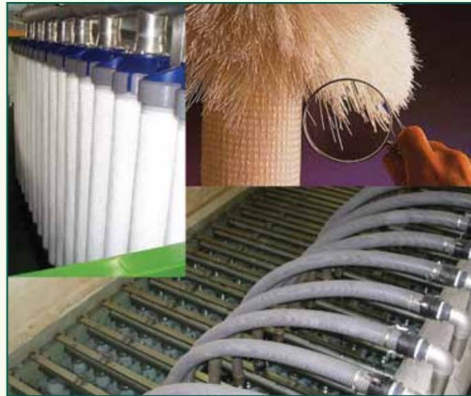
Clockwise: module rack, cut fibers, submerged membranes
