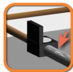
Service Line (also called distribution pipe ) Homeowners' pipes may be made of lead, copper, galvanized steel or plastic.
